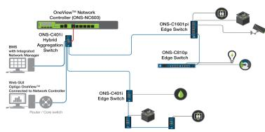
Hybrid connects networks running on copper, multimode, or mixed cabling networks. It's ideal for small networks and retrofit projects.
