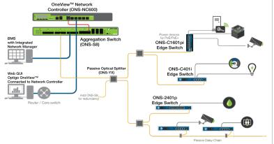
Spectra uses Passive Optical Networking to extend the reach of networks using single-mode fiber. It's perfect for large building networks and new build projects.
